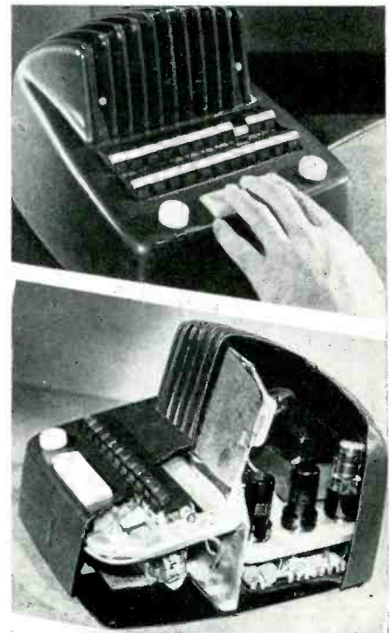
Top picture shows compact controls; lower cutaway shows details of construction and chassis of the Flexifone intercom control unit.
